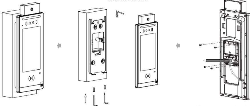
Installation is completed. And please remove the protective film.
