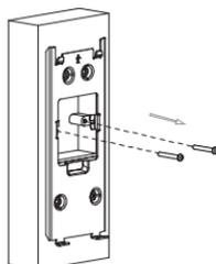
Remove the two M4x30 crosshead screw and take off the wall-mounting bracket.
