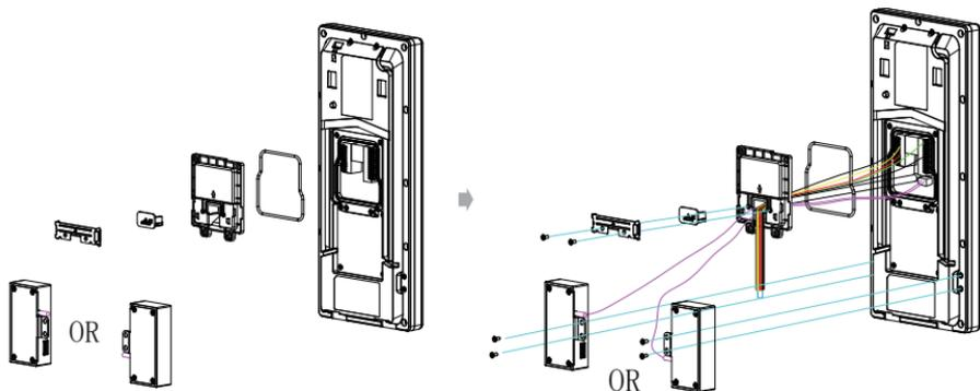
Take out the device and the digital wrist temperature detector and then take out wiring cover, sealing pressing plate, rubber plug, sealing ring and corresponding screws.
