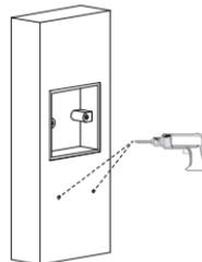
Use a hand drill with 6 mm diameter bit to make two positioning holes with 25 mm in depth in the marked positions.
