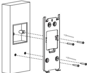
Fix the wall-mounting bracket with two M4x30 crosshead screw and two ST4x20 crosshead screw.
