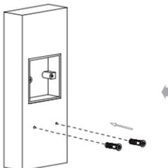
Insert two plastic wall anchors into the two drilled holes.
