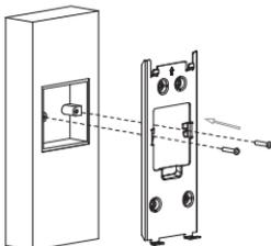
Fix the wall-mounting bracket on the embedded box with two M4x30 crosshead screw.
