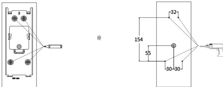
According to the position of the cable, put the wall-mounting bracket closely on to the wall and mark the four positioning holes, while making sure that relative positions between wall-mounting bracket and wire hole are correct.
