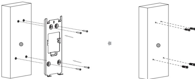
Fix the wall-mounting bracket with four ST4x20 crosshead screw.
