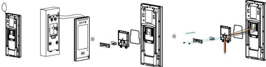
For convenient wiring, hang device on the wall-mounting bracket with rope.
