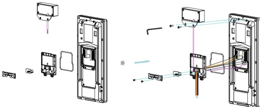
Take out the device and the digital forehead temperature detector and then take out wiring cover, sealing pressing plate, rubber plug, sealing ring and corresponding screws.
