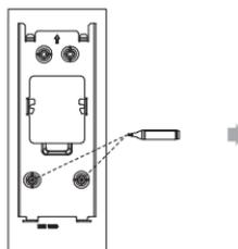
Mark the two positioning holes of the wall-mounting bracket on the wall.
